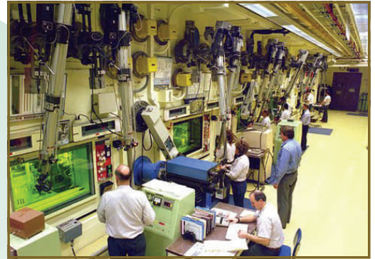
Engineers use robotic manipulators to perform Post-Irradiation Examination in hot cells at the Hot Fuel Examination Facility (HFEF) at INL.
