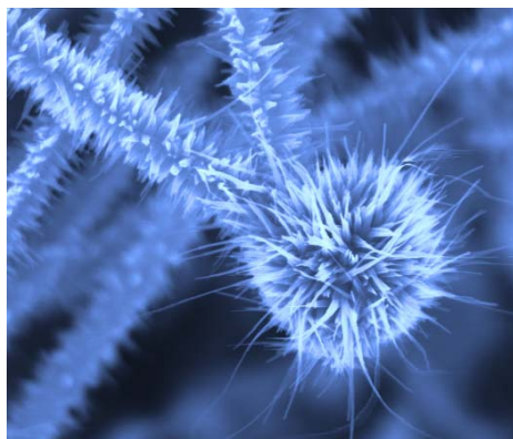
Cu-TCNQ nanowires on ZnO nanowires
